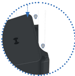
10 Tightening the head two bolts from above
